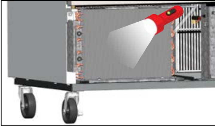
Fig. 5. Verify all blockages have been removed.
