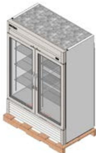
Fig. 1. Remove the exterior packaging.
