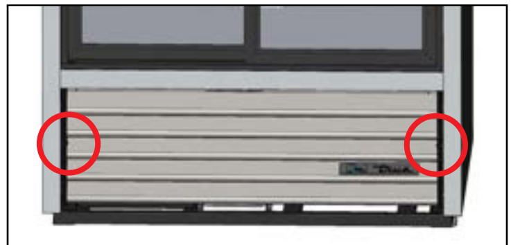
Fig. 2. Slide door louver grill screw locations.
