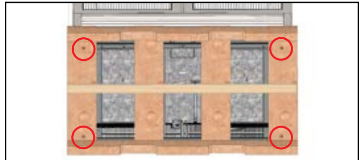
Fig. 4. Shipping bolt locations.
