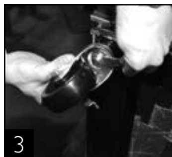
3 Use the tool provided to tighten the castor into place.
