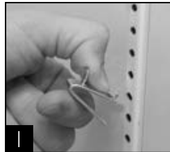
1 Installing top tab of shelf clip
